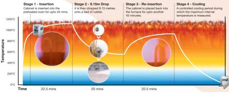
As the cabinet is affected by heat for a much longer time, the testing period can actually take up to 24 hours.
