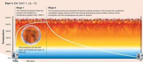
As the cabinet is affected by heat for a much longer time, the testing period can actually take up to 24 hours
